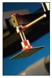
safely rework all types of components without overheating the component, adjacents or the PCB. It uses all the proven attributes of PDR's Focused IR technology, first introduced in 1987 and now used worldwide by over 4000 customers.
